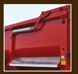
Double Hinge Tailgate Allows for hi-lift or free-flow action of tailgate.
