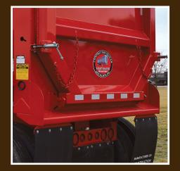
Spreader Apron Allows for more even spread of material during dump cycle.
