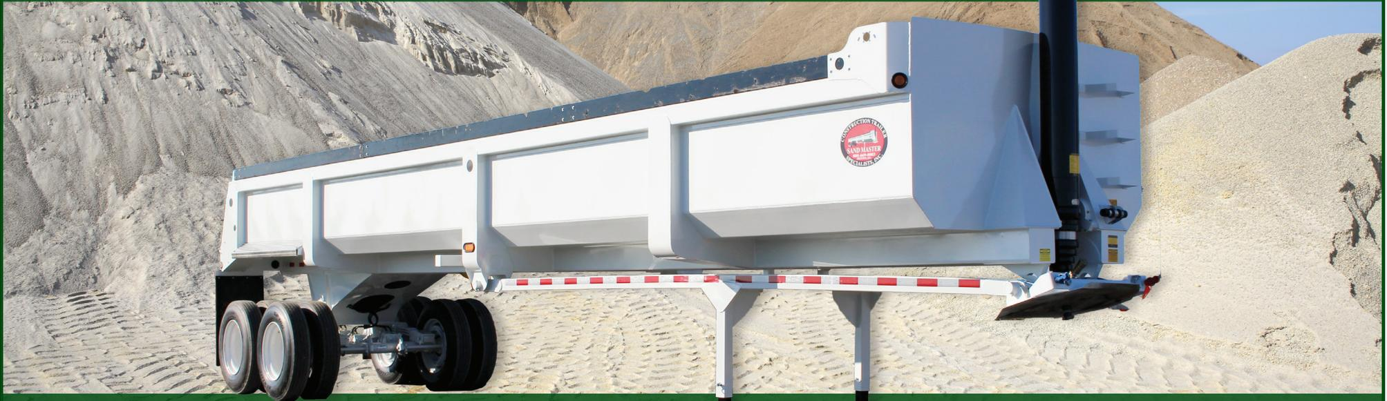
» Wear Plate Construction. No Liner Needed.
