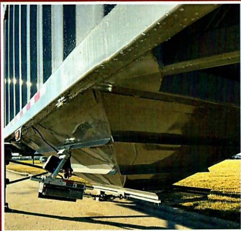
Electric Hopper Door Electrically Operated Hopper, Controlled by Push Button or Remote.
