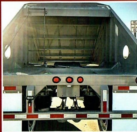
Walking Platform with Ladder Steel Walkway Platform with Ladder Access to Trailer Roof.
